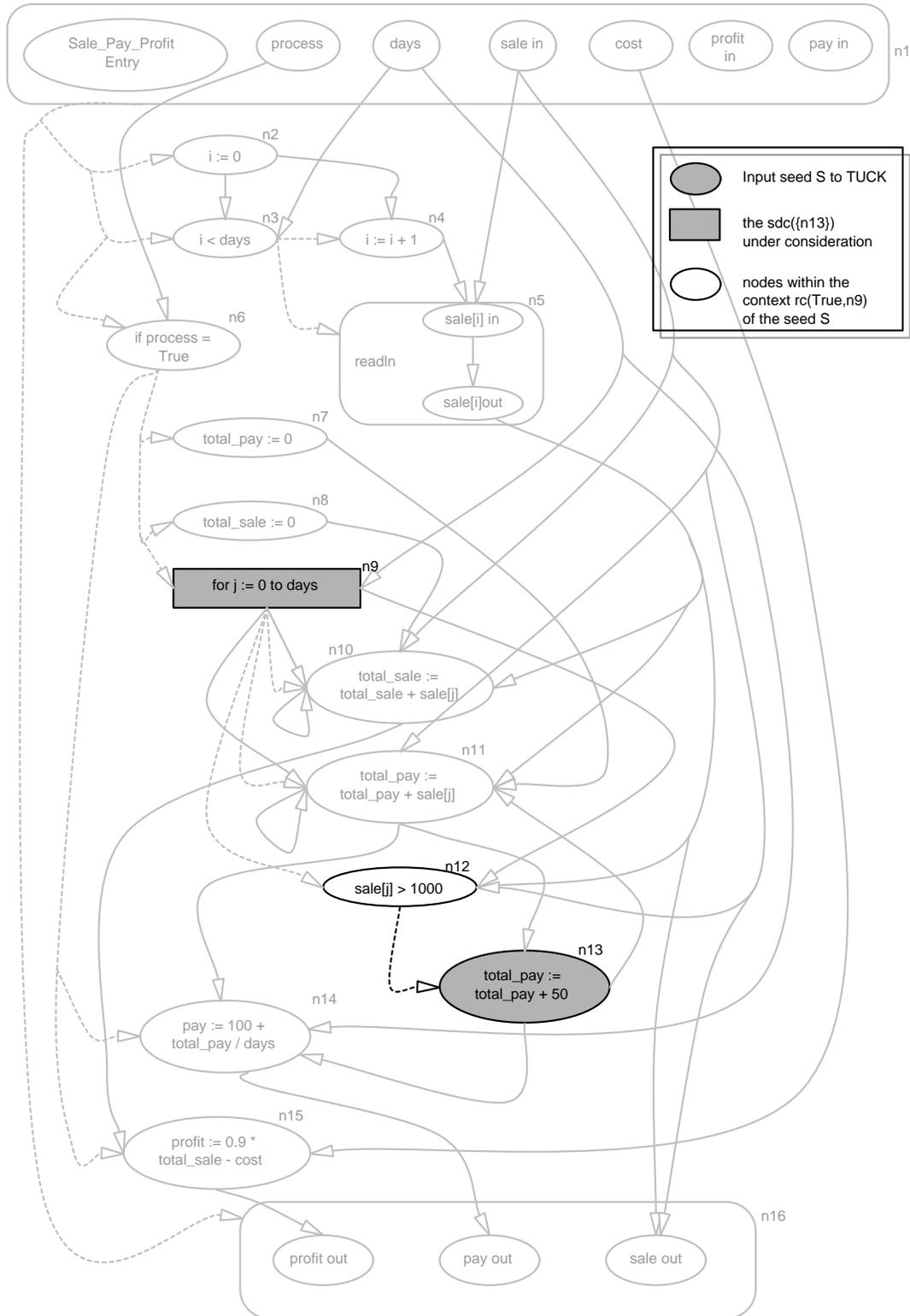
Figure 10:  $TUCK(n13)$  within the restructuring context defined by  $n9$ . The result of the slice within this context is  $\{n12, n13\}$ .
