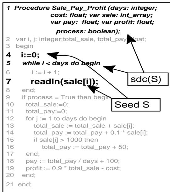
Figure 14 : TUCK first identifies all the single definite control of the seed S.
