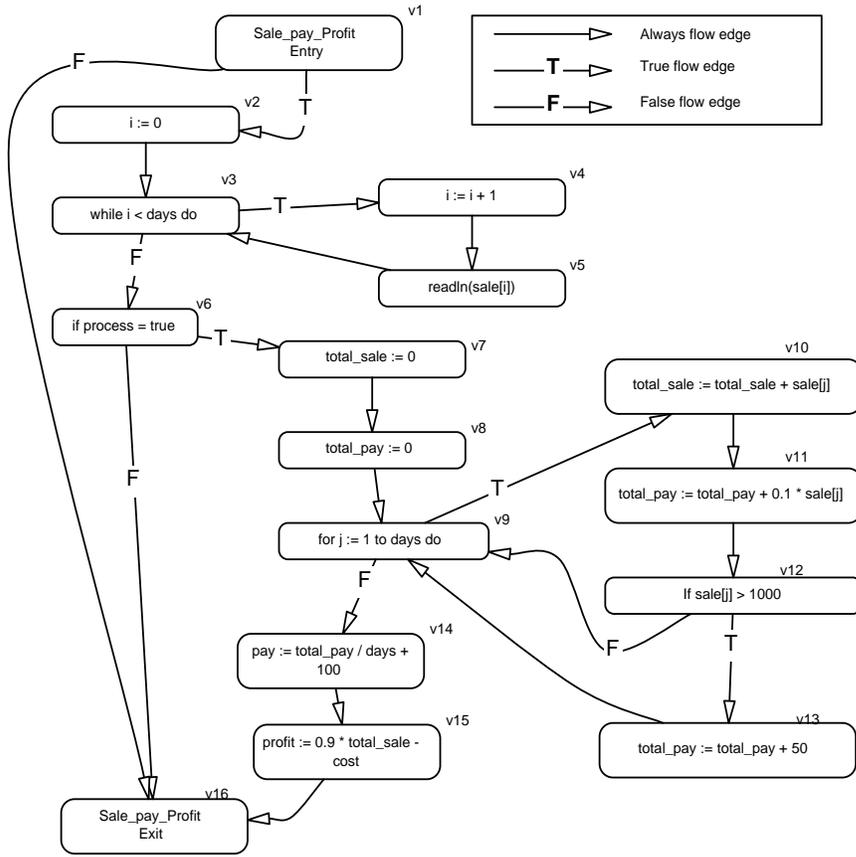
Figure 4: CFG for Sale\_Pay\_Profit procedure of Figure 1.
